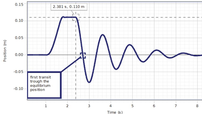
Figure 2 - Cart position vs. time, showing damped oscillation. The initial position of the oscillator (0.110 m) is evidenced.
