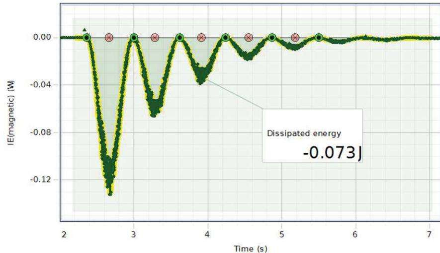
One may wonder again if it is possible to recover another simple result: the energy dissipated should be given by the value of the energy initially stored in the springs:
