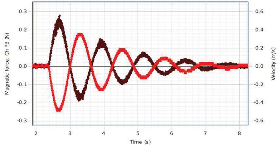
The force of the magnets on the cart is proportional to the velocity but with opposite sign (Fig. 4). This agrees with the assumption that the magnetic force is of viscous type. We now discuss the energy flows as functions of time. At first, we consider the interaction between cart and springs shown in Fig. 5.
