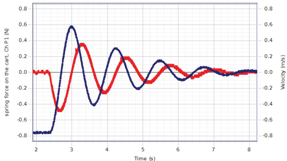
Since the velocity is zero at the turning points and has a maximum when the cart transits through the equilibrium position, we understand why measurements show a shift of a quarter of a period between the velocity and the spring force (in Fig. 3, only the velocity and the force on the cart exerted by the spring on the left, measured by sensor  $F_1$ , are displayed).
