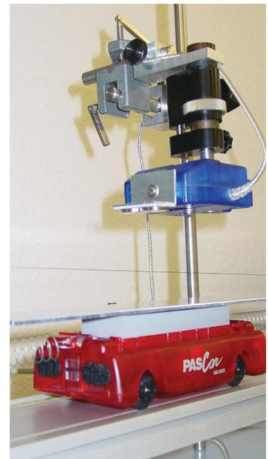
Figure 1 – Kinematic data is taken by a rotary motion sensor (RMS). The springs are fixed to two force sensors ( $F_1$  and  $F_2$ ). The magnets responsible for the dissipative interaction are attached to a third force sensor ( $F_3$ ) allowing to determine the horizontal value of the damping force on the cart.
