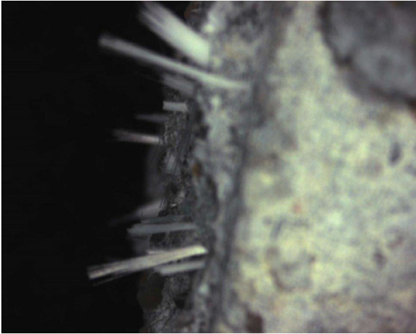
Figure 4. Images (obtained from the optical microscope) of lateral view of the failure surface of sample G3%_03.
