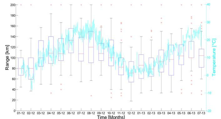
Figure 3: boxplot of the estimated range in function of the temperature
