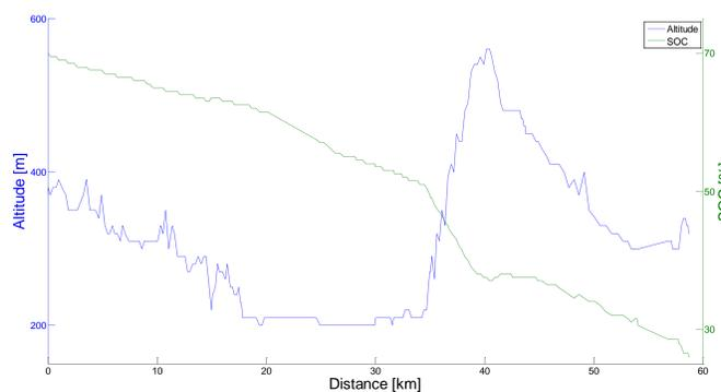
Figure 1: trend of the SOC in a typical travel with relative territory profile
