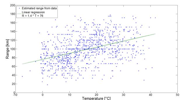
Figure 4: dispersion of the estimated range data in function of the temperature
