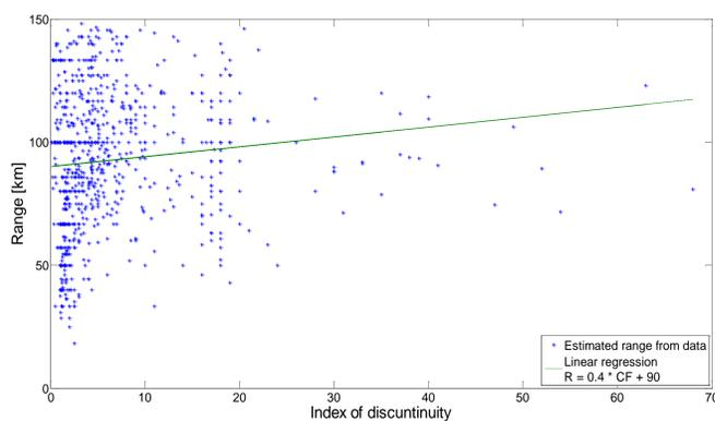
Figure 2: estimated range in function of the index of discontinuity
