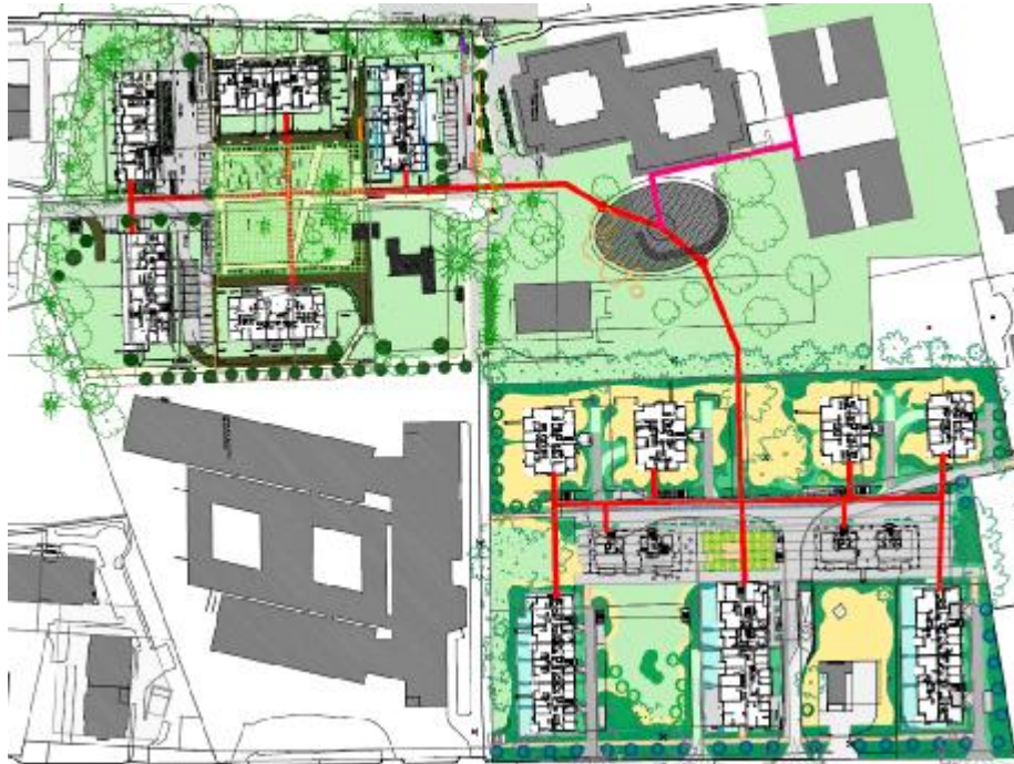
Figure 1 Configuration: Florence (9 buildings), Champendal (5 buildings), solar collectors on the flat roofs of the school located near the oval ground storage
