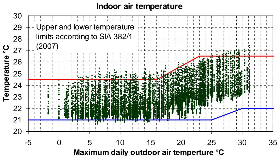
Abb. 4: Simulated indoor air temperature for the building reference case.
