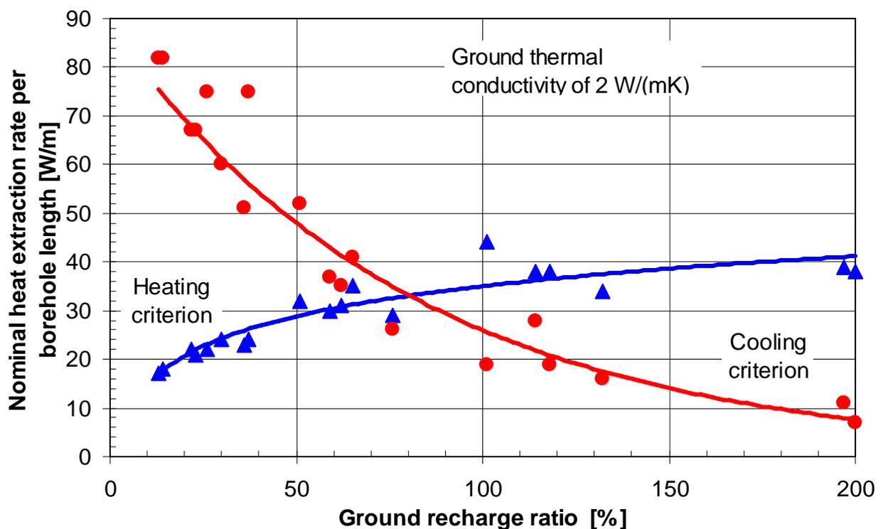
Abb. 6: Influence of the ground recharge ratio on the system design. The borehole length is expressed in terms of nominal heat extraction rate of the heat pump, both for the heating and cooling criteria. The nominal power of the heat pump is adapted from case to case according to the building design and climatic data.
