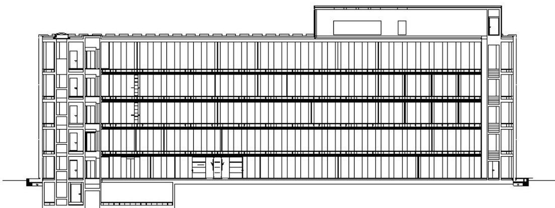
Abb. 3: East-west cross section of the Chiasso-Brogeda building used for the definition of the reference building.
