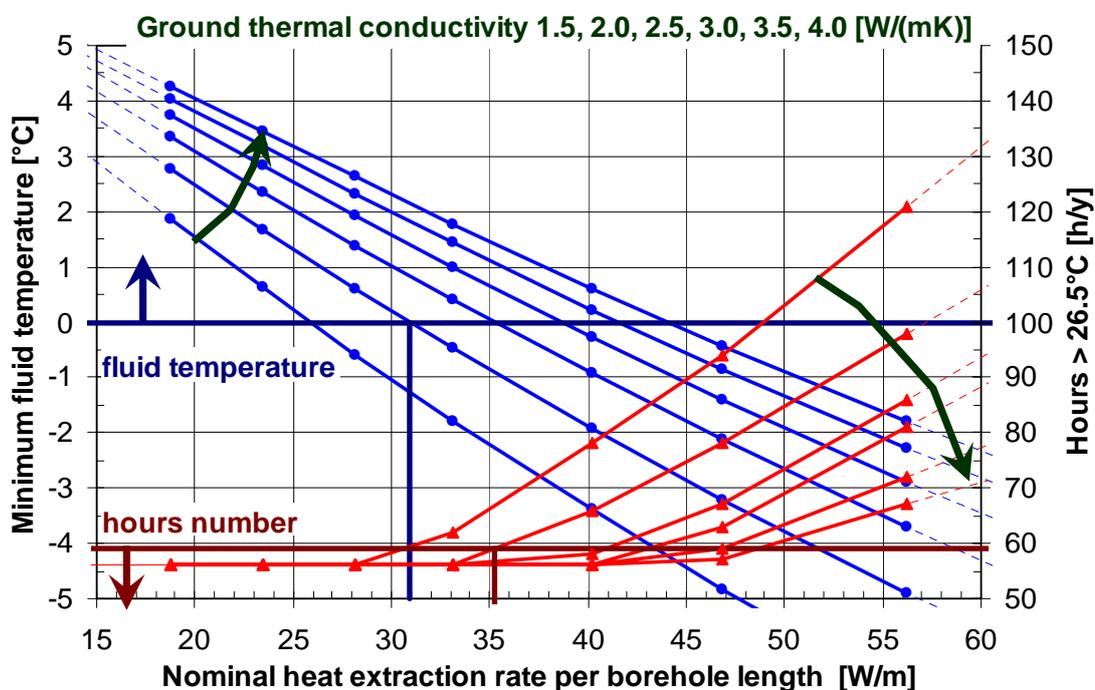
Abb. 5: Influence of the ground thermal conductivity on the system design. The borehole length is expressed in terms of nominal heat extraction rate of the heat pump, both for the heating and cooling criteria.
