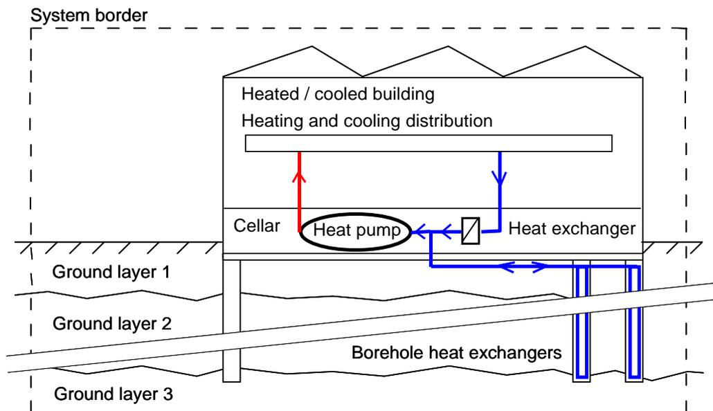
Abb. 2: The system simulated by COOLSIM, the TRNSED application of TRNSYS, is indicated by the system border.
