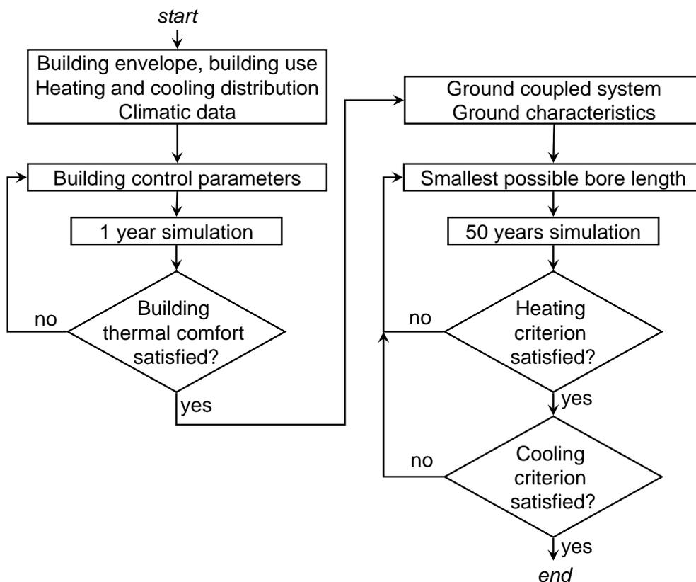
Abb. 1: Followed methodology for the determination of an optimal system design for a ground coupled system.
