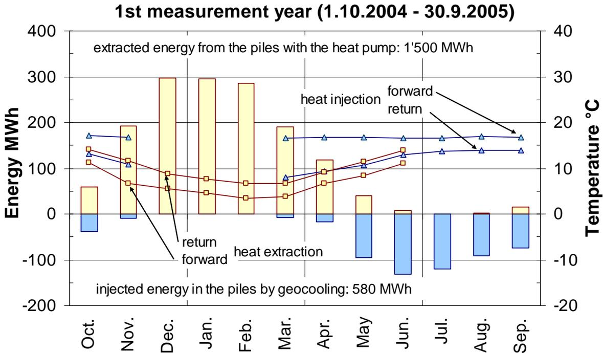
Figure 5: Monthly extracted and injected energies in the piles. The monthly temperature levels of the heat carrier fluid in the pile circuit are shown for both the extraction and injection operation modes
