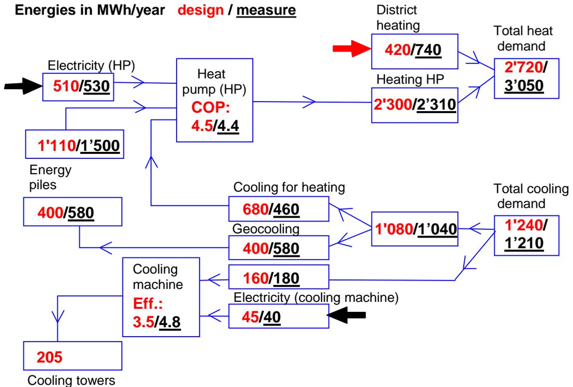
Figure 7: Pile system heat balance, comparison measured – predicted values with PILESIM
