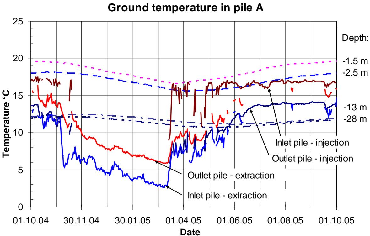
Figure 6: Ground temperatures in pile A at various depths. Daily temperature levels of the heat carrier fluid in the pile circuit are shown for both the extraction and injection operation modes
