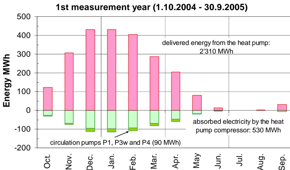
Figure 3: Monthly thermal performances of the heat pump
