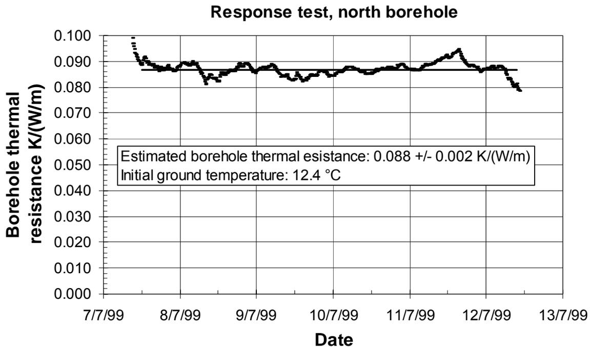
Fig. 7 Estimation of the effective borehole thermal resistance of the north borehole.
