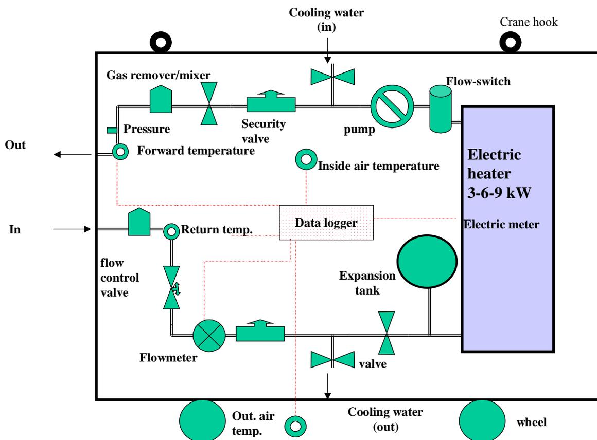
Fig. 2 Schematic view of the response test device.
