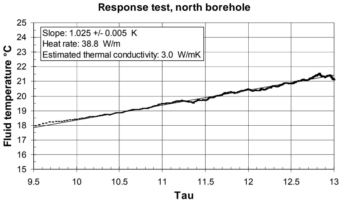
Fig. 6 Estimation of the thermal conductivity for the north borehole.
