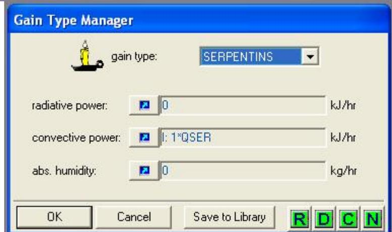
Figure 6.7 Input parameters in TRNBuild for the definition of the input convective heat gain in the zone PONT
