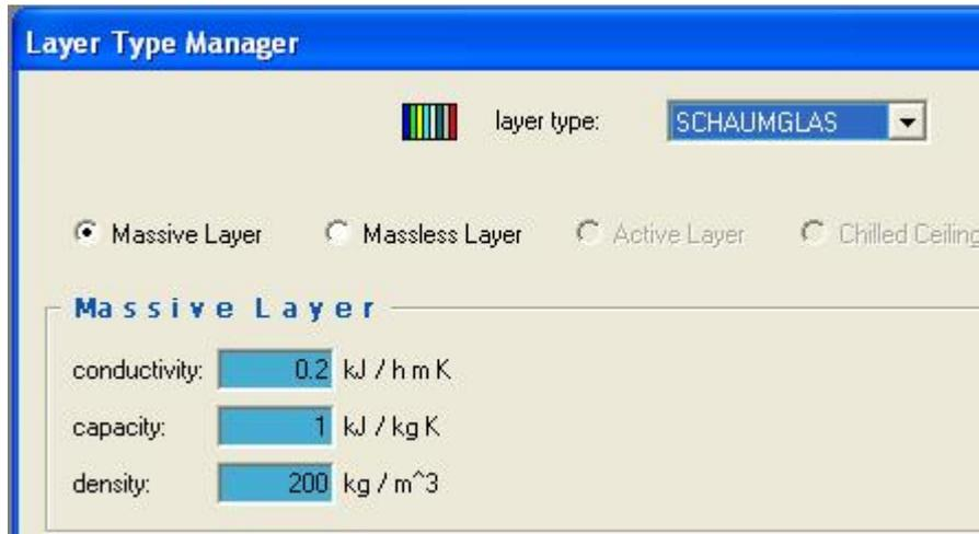
Figure 6.6 *Input parameters in TRNBuild for the thermal characteristics of the various material layers*
