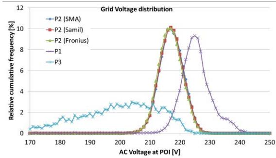
Figure 4: Grid voltage distribution in the three locations (P1, P2, P3)
