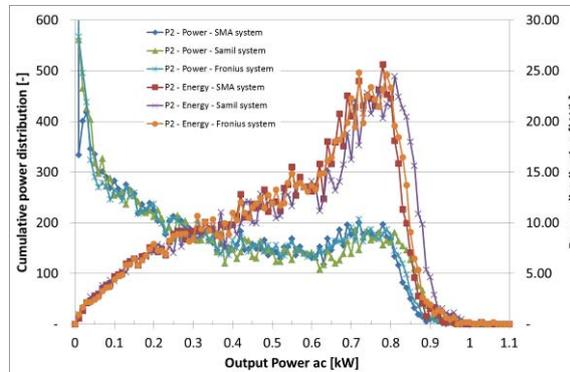
Figure 8: Power and energy distribution at the P2 Nepal reference location in the NEA Min Bhawan Office, Kathmandu.
