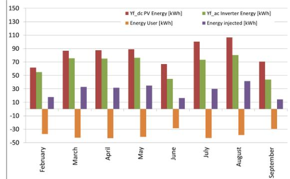
Figure 9: dc final yield, ac final yield, losses during load shedding events, energy used and energy injected into the grid in location P1, CES/IOE Tribhuvan University, Kathmandu, Nepal.
