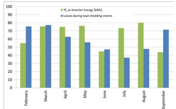
Figure 10: Energy production (Yf\_ac final yield) and calculated losses during load shedding events; location P1.
