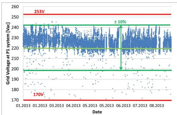
Figure 5: Grid voltage variation during the selected period of analysis of the P1 PV system, at POI.
