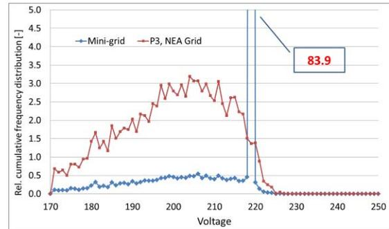
Figure 6: Relative frequency distribution of voltage at the P3 power plant operating in grid connected mode (red) and with Mini-grid mode (Blue).
