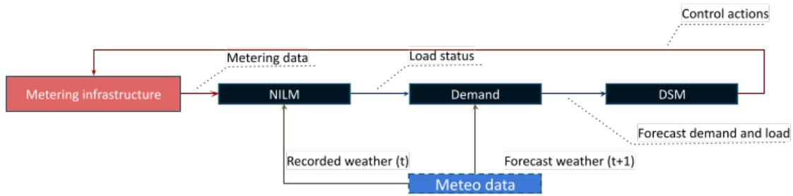
**Figure 1:** Schematic representation of Optiflex.
