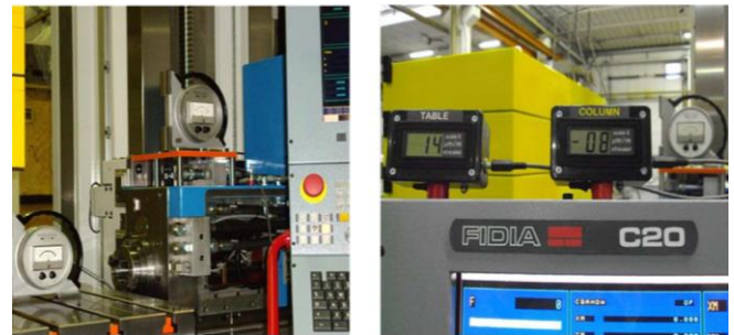
Fig. 14: Inclinometers used to measure roll and pitch
