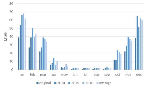
Figure 7. Kindergarten “H.C. Andersen”: energy consumption simulation of in the original situation and during the following three year of operation phase.
