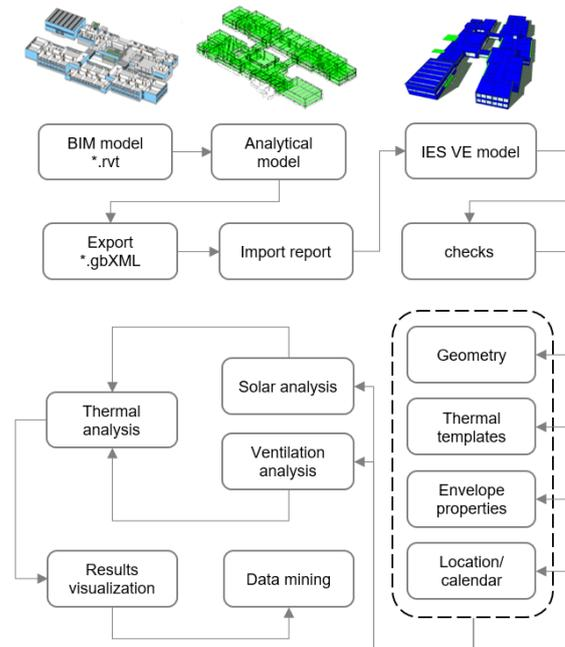
Figure 1. Workflow for interoperability BIM2BEM.
