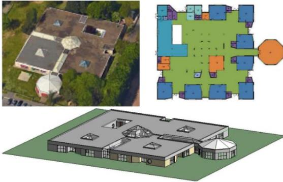
Figure 4. Aerial view of the kindergarten "H.C. Andersen", floor area with functional spaces and BIM model.
