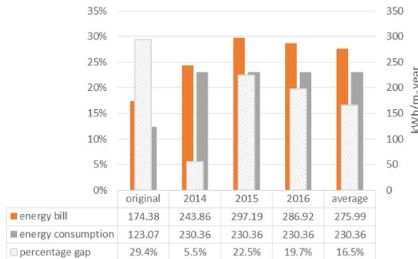
Figure 8. Kindergarten "H.C. Andersen": actual energy bills compared to energy consumption simulation and the percentage gap between simulation and real data.
