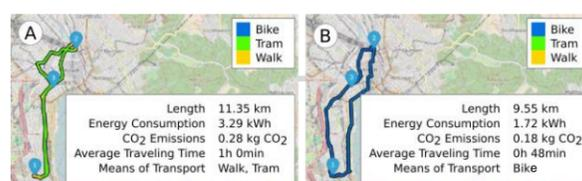
Figure 1 A systematic loop (A) and the ecological alternative we computed (B).
