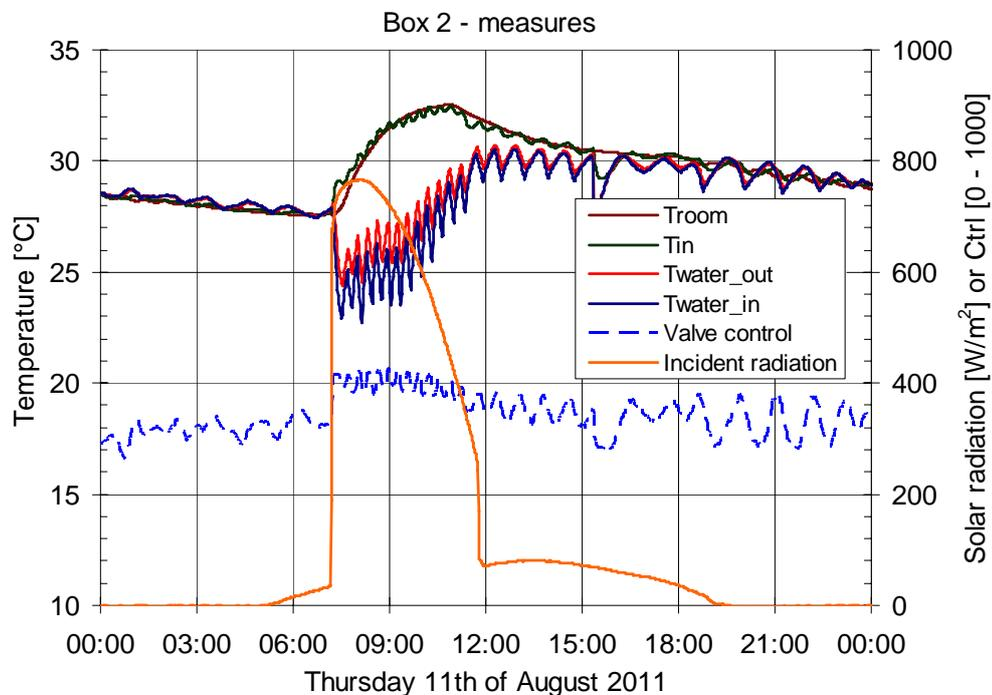
Figure 2 Typical measurements with the PID controller regulating the inside air temperature of the box ( $T_{in}$ ) on the room air temperature ( $T_{room}$ )
