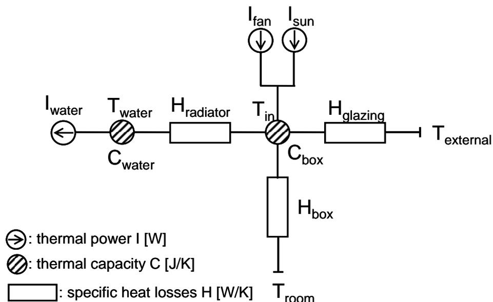
Figure 1 Simplified thermal model of a box with two temperature nodes
