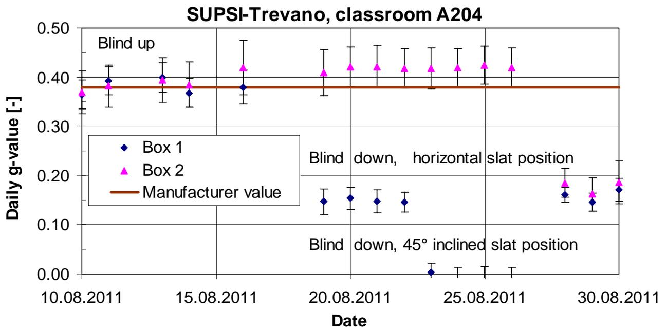
Figure 7 Daily g-value measured in the classroom A204 of SUPSI in Lugano-Trevano. Three positions of the blinds are tested: blind up, blind down with horizontal slat position and blind down with  $45^\circ$  inclined slat position
