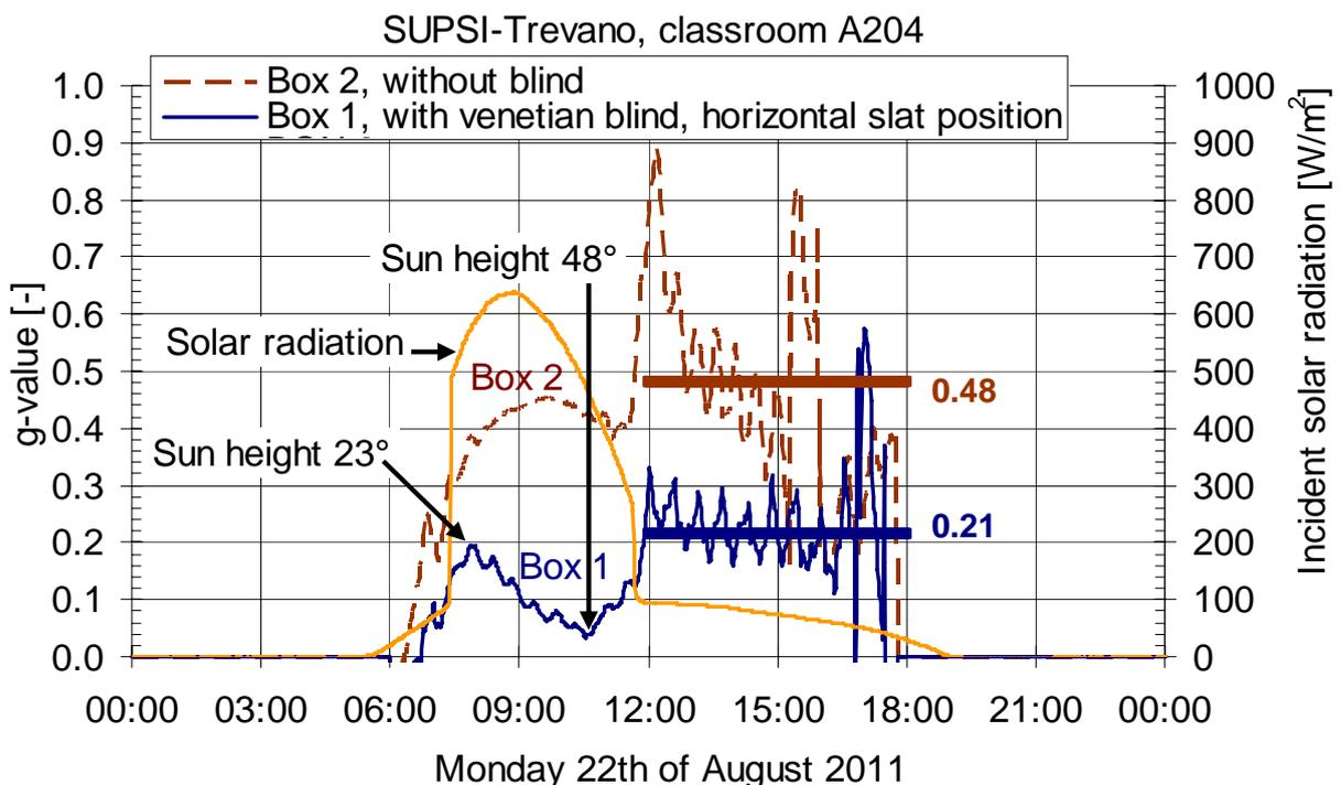
Figure 6 Evolution of the measured g-value for a clear sunny day in Lugano. A triple glazing with an external venetian blind is measured by Box 1. Box 2 report the measured g-value of the triple glazing without solar protection
