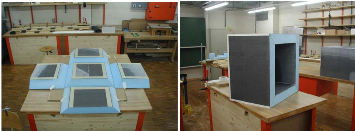
Figure 4: Assembly of prototype calorimeter
