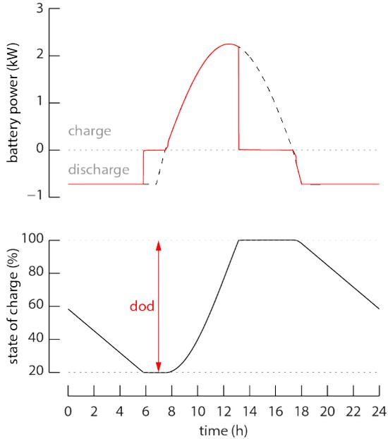
**Figure 3:** Example of battery control system behavior
