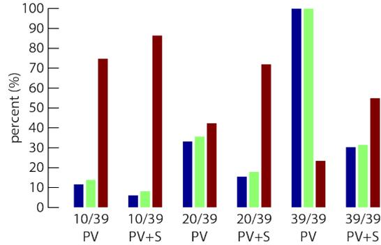
**Figure 5:** Simulations results: Blue: Relative instability of transformer power, green: relative median instability of local V, red: neighborhood self-consumption.
