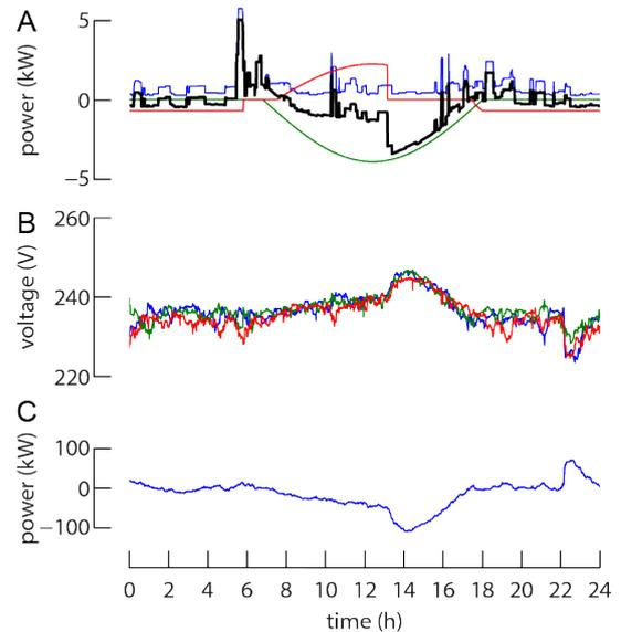
**Figure 4:** Example of simulation. A: household power consumption. Blue: uncontrolled loads, green: PV, red: battery, black: total. B: Voltage and the main panel for the three phases. Blue: phase 1, green: phase 2, red: phase 3. C: total power consumption at the LV transformer.
