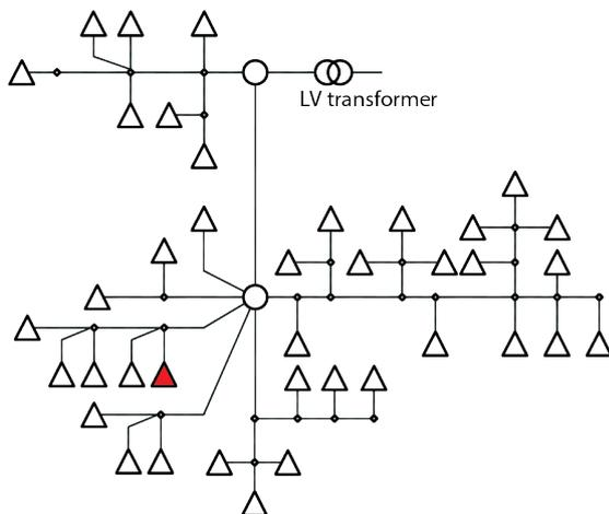
**Figure 1:** Layout of the modeled low voltage distribution grid branch. Triangles: houses, circles: electrical cabinets. The red house denotes the position of the example case of figure 4.
