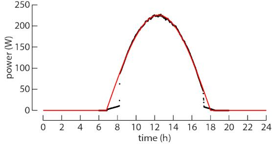
**Figure 2:** PV power's trend during a VERY CLEAR day (black dots) and its sine fit (red line).
