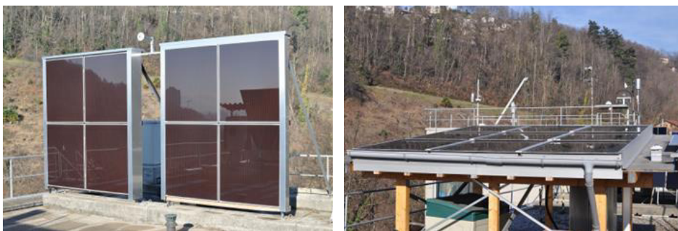
Fig. 2: Two vertical façades and a roof top BIPV installation are compared with reference free-standing modules.
