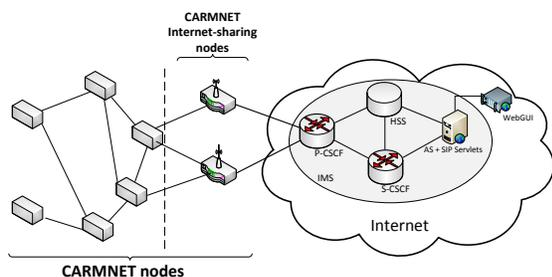
Fig. 2: The CARMNET system general architecture.
