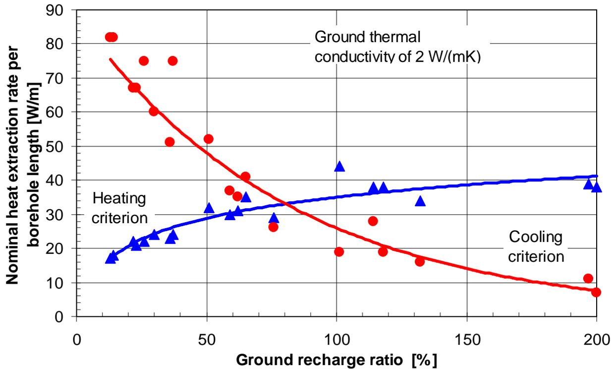
Figure 6 : Influence of the ground recharge ratio on the system design. The borehole length is expressed in terms of nominal heat extraction rate of the heat pump, both for the heating and cooling criteria. The nominal power of the heat pump is adapted from case to case according to the building design and climatic data.
