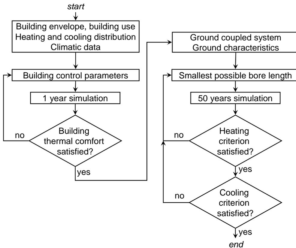
Figure 1 : Followed methodology for the determination of an optimal system design for a ground coupled system.
