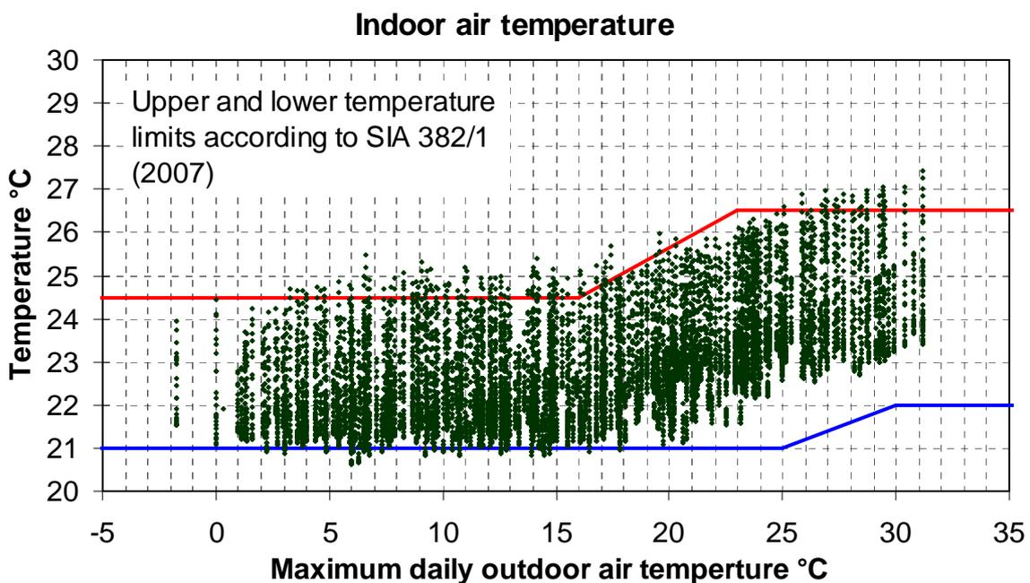
Figure 4 : Simulated indoor air temperature for the building reference case.
