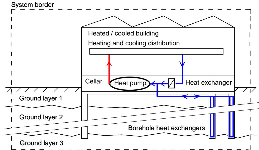
Figure 2 : The system simulated by COOLSIM, the TRNSED application of TRNSYS, is indicated by the system border.
