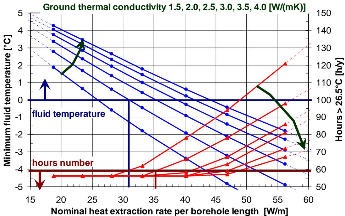
Figure 5 : Influence of the ground thermal conductivity on the system design. The borehole length is expressed in terms of nominal heat extraction rate of the heat pump, both for the heating and cooling criteria.
