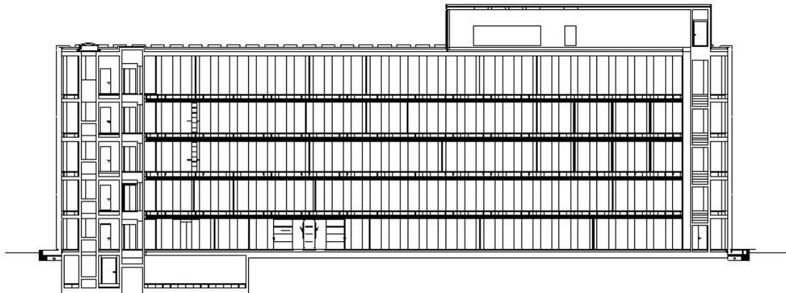
Figure 3 : East-west cross section of the Chiasso-Brogeda building used for the definition of the reference building.
