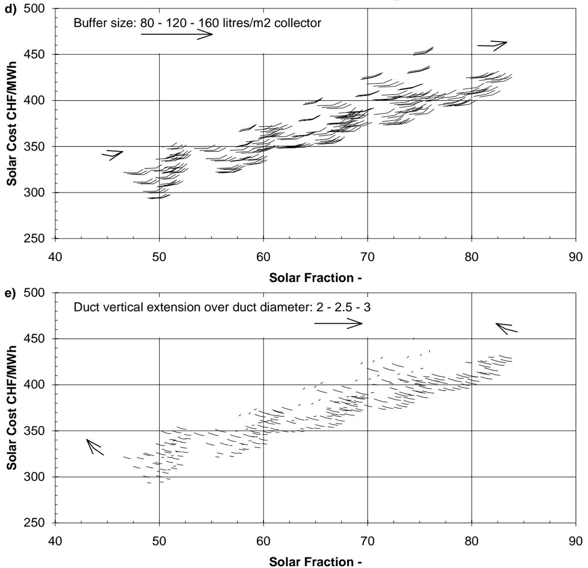
Fig. 8.5d-e: Medium heat load, 1'000 MWh/y (50% space heating and 50% domestic hot water); moderate-temperature heat distribution.
