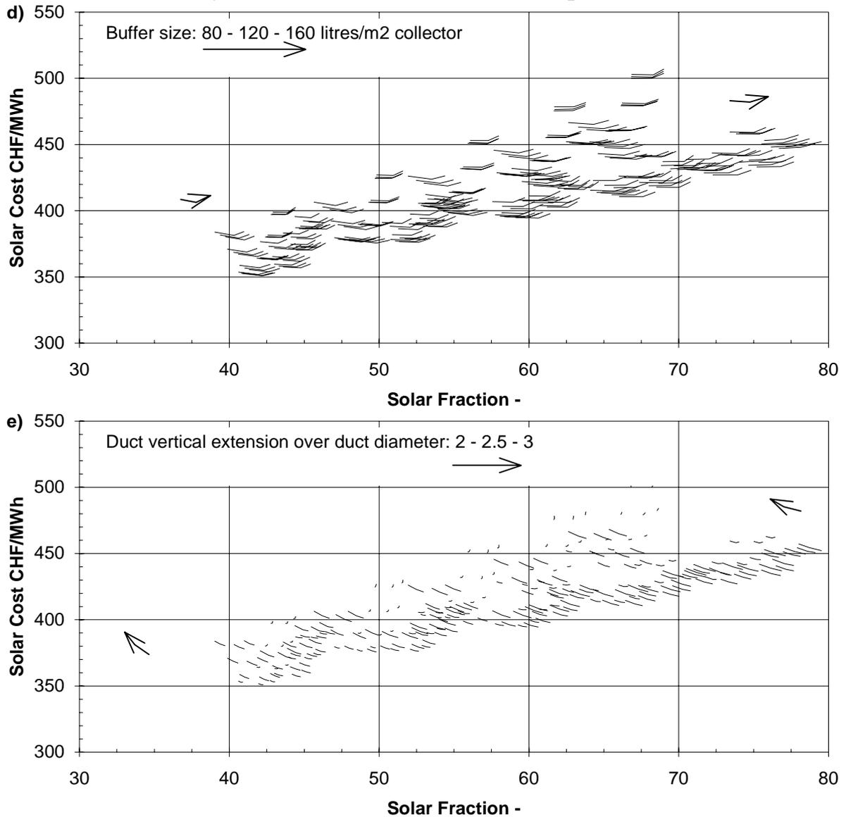
Fig. 8.2d-e: Medium heat load, 1'000 MWh/y (75% space heating and 25% domestic hot water); moderate-temperature heat distribution.
