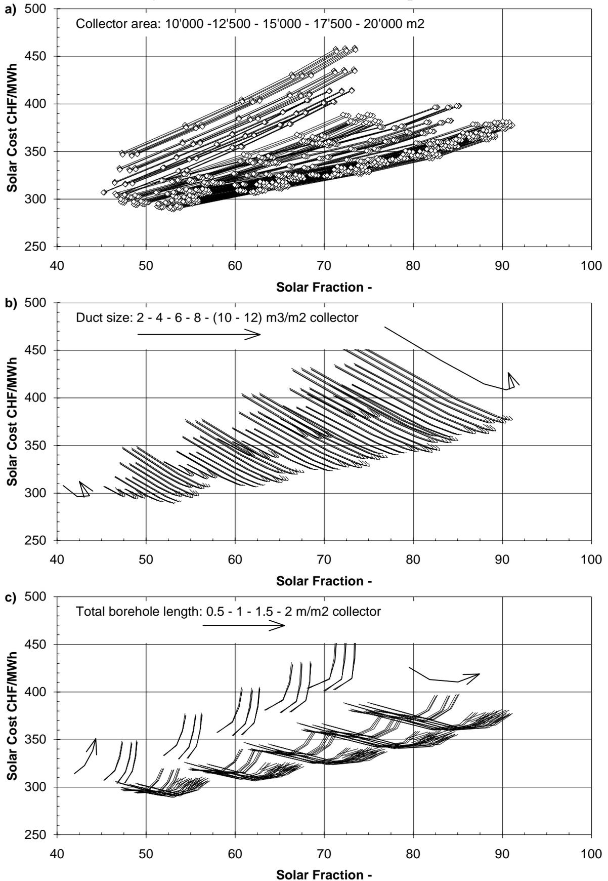
Fig. 8.3a-c: Large heat load, 5'000 MWh/y (75% space heating and 25% domestic hot water); moderate-temperature heat distribution.
