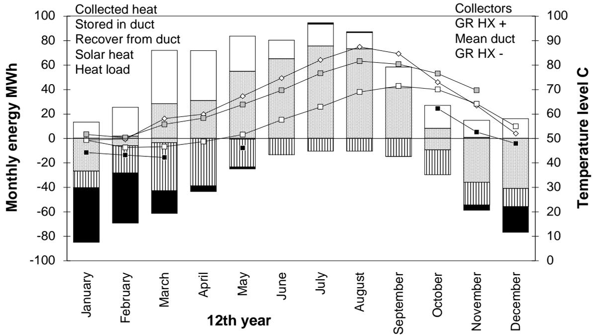
Fig. 8.10: Monthly heat balance of the system designed for the S75MOD load type; (small heat load, 500 MWh/y, 75% space heating and 25% domestic hot water, moderate-temperature heat distribution). The solar fraction corresponds to approximately 70%.
