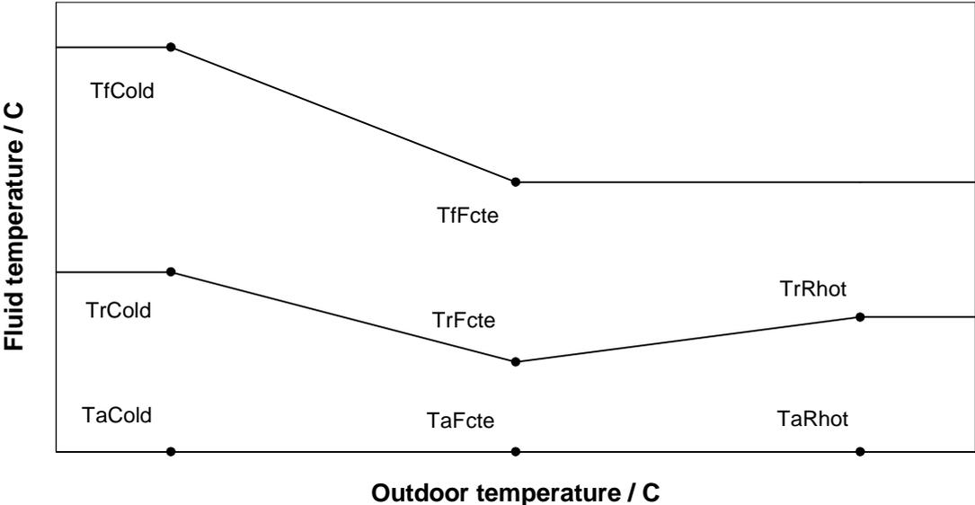
Fig. A4.2 The forward and return fluid temperatures in the distribution network are prescribed and depend on the outdoor air temperature.
