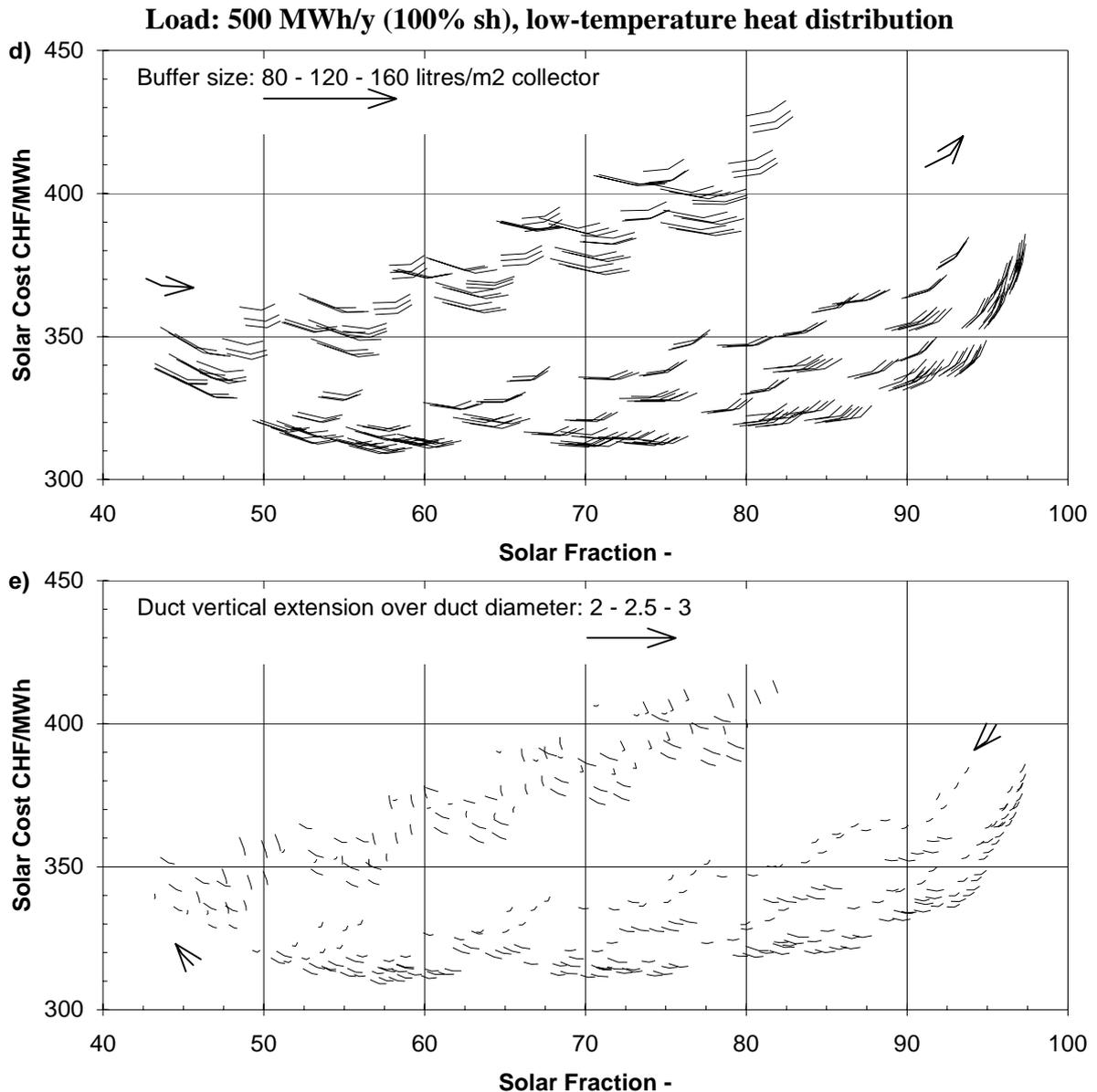
Fig. 8.7d-e: Small heat load, 500 MWh/y (100% space heating); low-temperature heat distribution.
