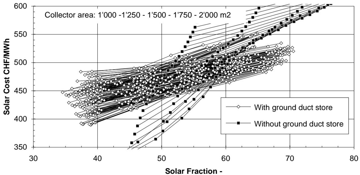
Fig. 8.8: Small heat load, 500 MWh/y (75% space heating and 25% domestic hot water); moderate-temperature heat distribution. Comparison of the solar cost for systems with or without ground duct store, in addition to a water store.
