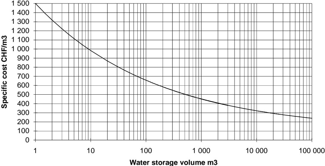
Fig. 4.1 Specific cost of an installed water tank store shown in relation to the tank volume.
