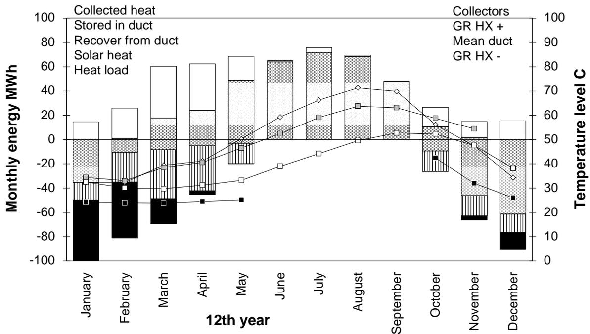
Fig. 8.12: Monthly heat balance of the system designed for the S100LOW load type; (small heat load, 500 MWh/y, 100% space heating, moderate-temperature heat distribution). The solar fraction corresponds to approximately 70%.
