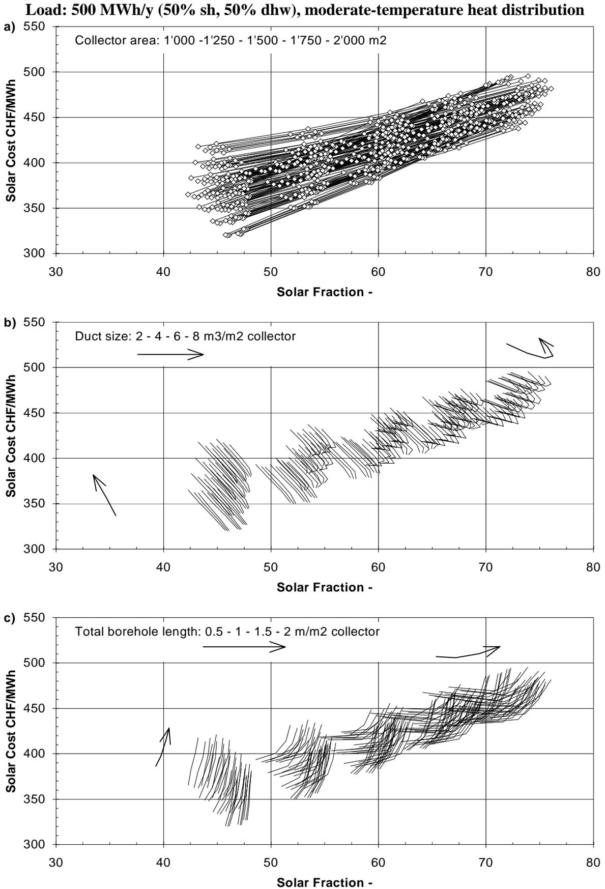
Fig. 8.4a-c: Small heat load, 500 MWh/y (50% space heating and 50% domestic hot water); moderate-temperature heat distribution.
