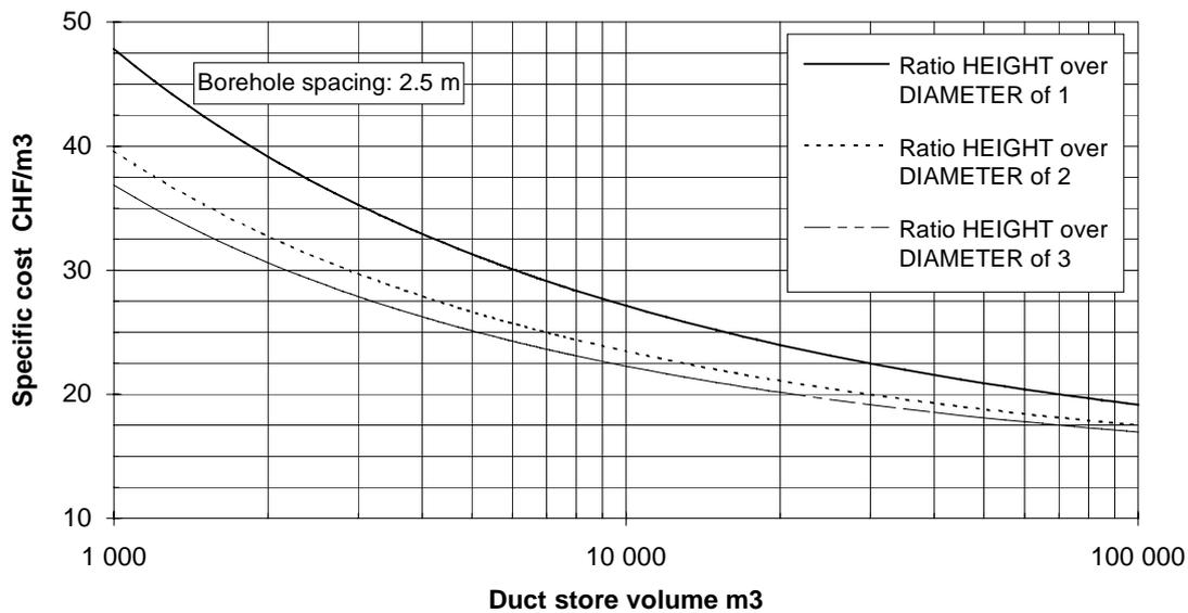
Fig. 4.2 Specific cost of a duct store shown in relation to the tank volume. The cost is calculated for 3 different shapes of the store, defined with the ratio HEIGHT over DIAMETER. The diameter is defined as the diameter of the disk whose area is the same as the store section. The borehole spacing is set to 2.5 m; a layer of 20 cm of insulation covers the top of the store and extends to 5% of its vertical extension; the top of the store is at the ground surface.
