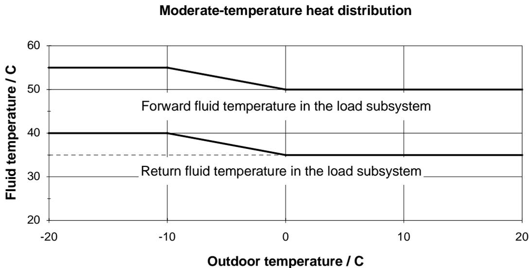
Fig. 5.1 Forward and return fluid temperature defining the moderate-temperature heat distribution.
