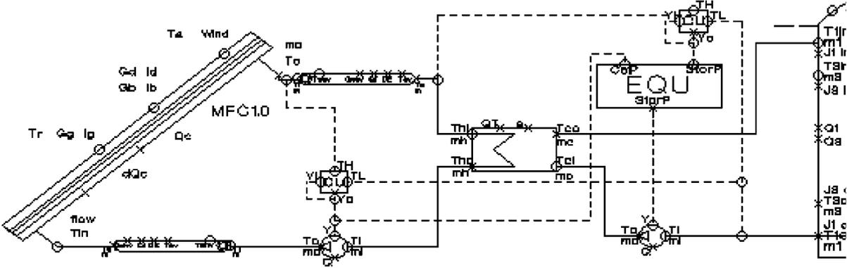
Fig. A6.1 Collector subsystem simulated with two pipes and two controllers.
