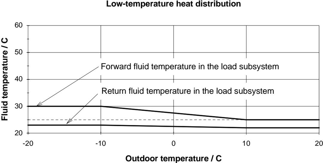
Fig. 5.2 Forward and return fluid temperatures defining the low-temperature heat distribution.
