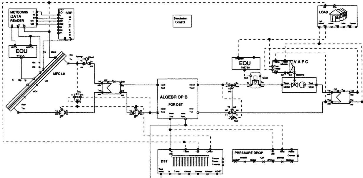
Fig. 6.2. PRESIM representation of the system design without a short-term buffer tank.
