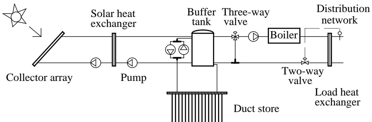
Fig 3.2 Design of the system with a short-term buffer tank.
