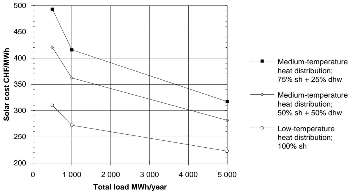
Fig. 8.9: Solar cost of the systems for the three kind of heat loads shown in relation to the load size. An annuity factor of 0.1 is assumed in the calculation of the solar cost.
