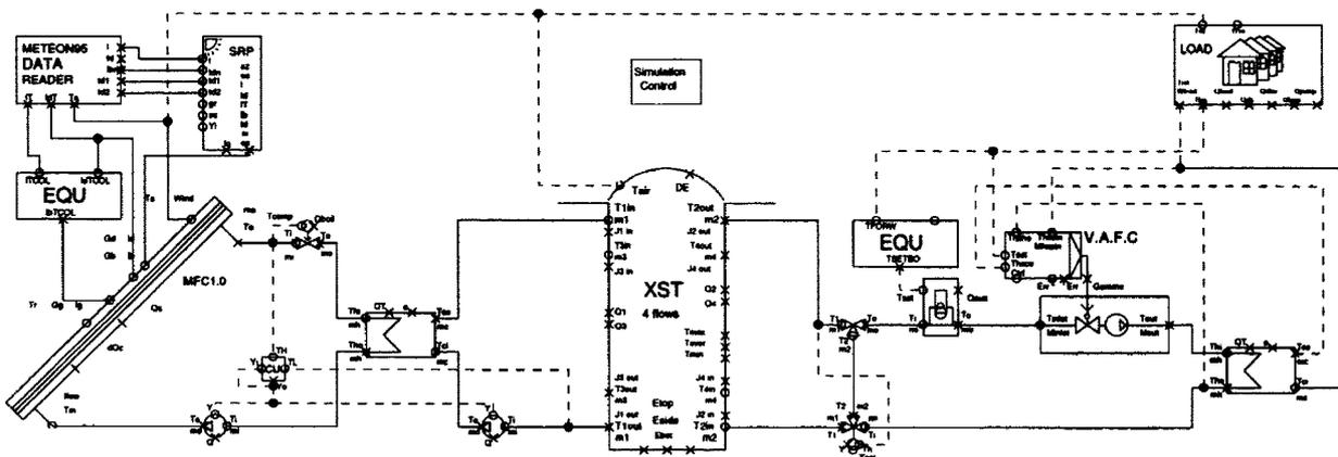
Fig. 6.3. PRESIM representation of the system design without a duct store.
