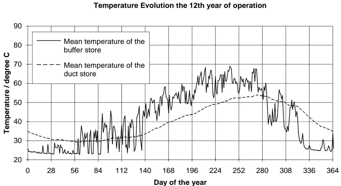
Fig. 8.13: Evolution of the mean temperature of the buffer and duct store. The simulated temperatures correspond to the system designed for the S100LOW load type; (small heat load, 500 MWh/y, 100% space heating, low-temperature heat distribution).
