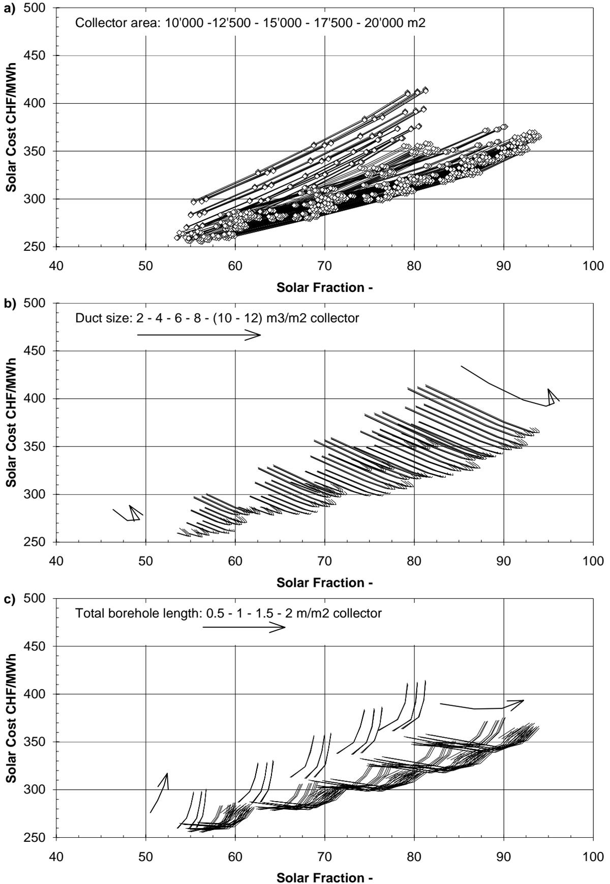
Fig. 8.6a-c: Large heat load, 5'000 MWh/y (50% space heating and 50% domestic hot water); moderate-temperature heat distribution.
