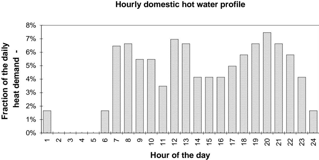
Fig. A4.1 Hourly profile of the domestic hot water heat demand. The hourly values are shown as a fraction of the daily heat requirement.
