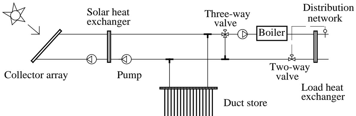
Fig 3.1 Design of the system without a short-term buffer tank.
