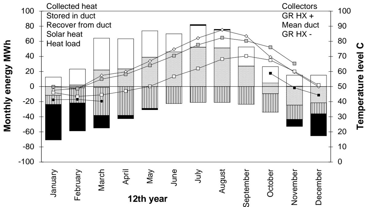
Fig. 8.11: Monthly heat balance of the system designed for the S50MOD load type; (small heat load, 500 MWh/y, 50% space heating and 50% domestic hot water, moderate-temperature heat distribution). The solar fraction corresponds to approximately 70%.
