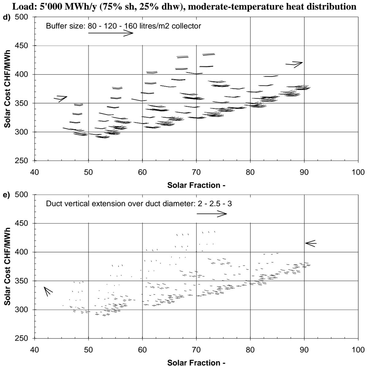
Fig. 8.3d-e: Large heat load, 5'000 MWh/y (75% space heating and 25% domestic hot water); moderate-temperature heat distribution.
