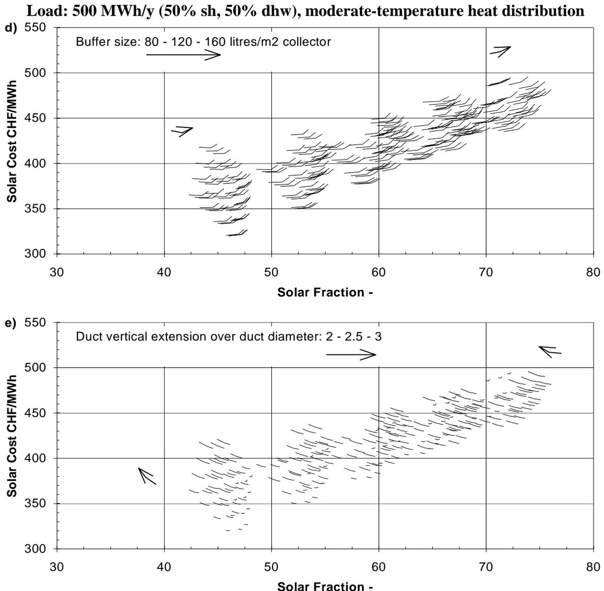
Fig. 8.4d-e: Small heat load, 500 MWh/y (50% space heating and 50% domestic hot water); moderate-temperature heat distribution.
