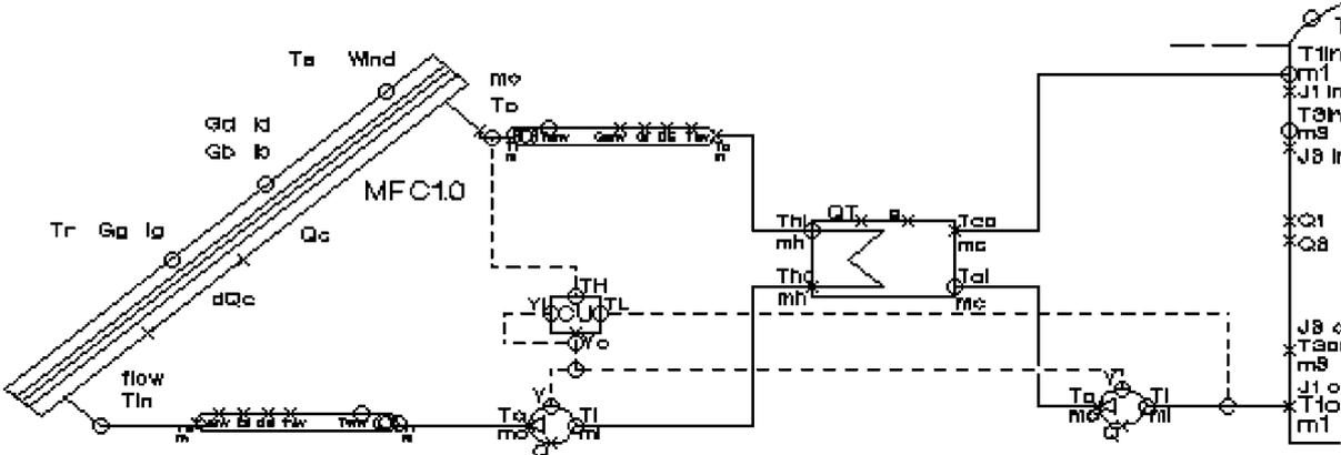
Fig. A6.2 Collector subsystem simulated with two pipes and one controller.
