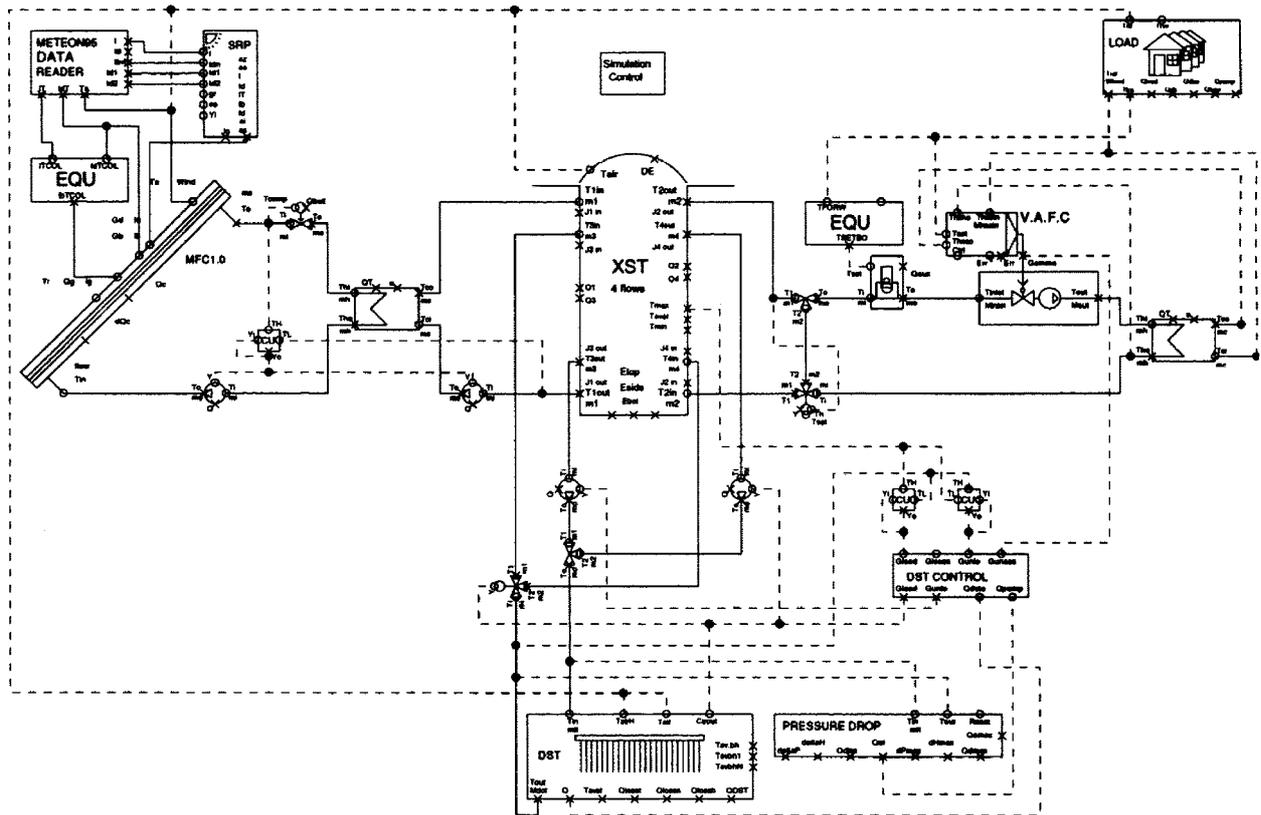
Fig. 6.1. PRESIM representation of the system design with a short-term buffer tank.
