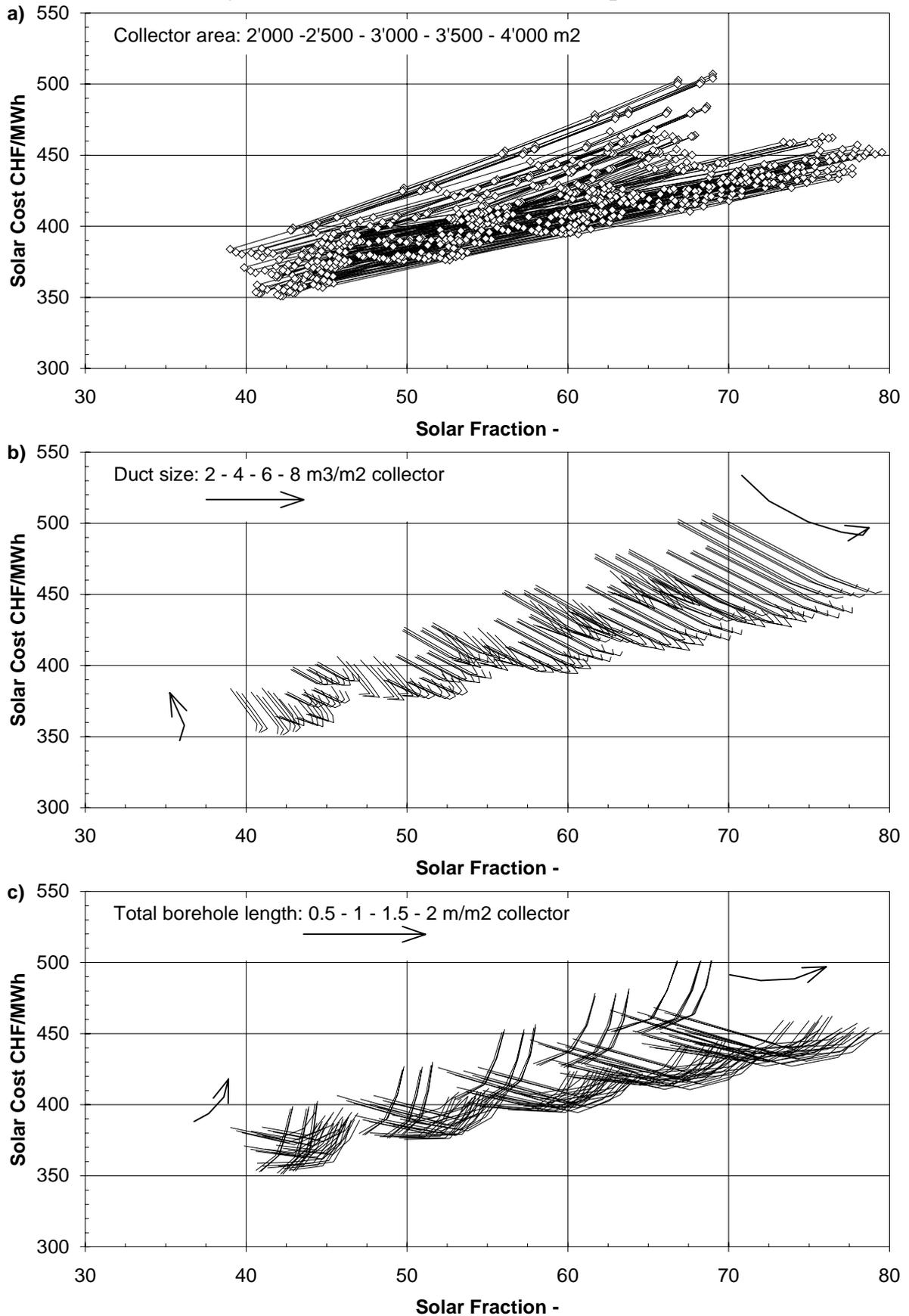
Fig. 8.2a-c: Medium heat load, 1'000 MWh/y (75% space heating and 25% domestic hot water); moderate-temperature heat distribution.
