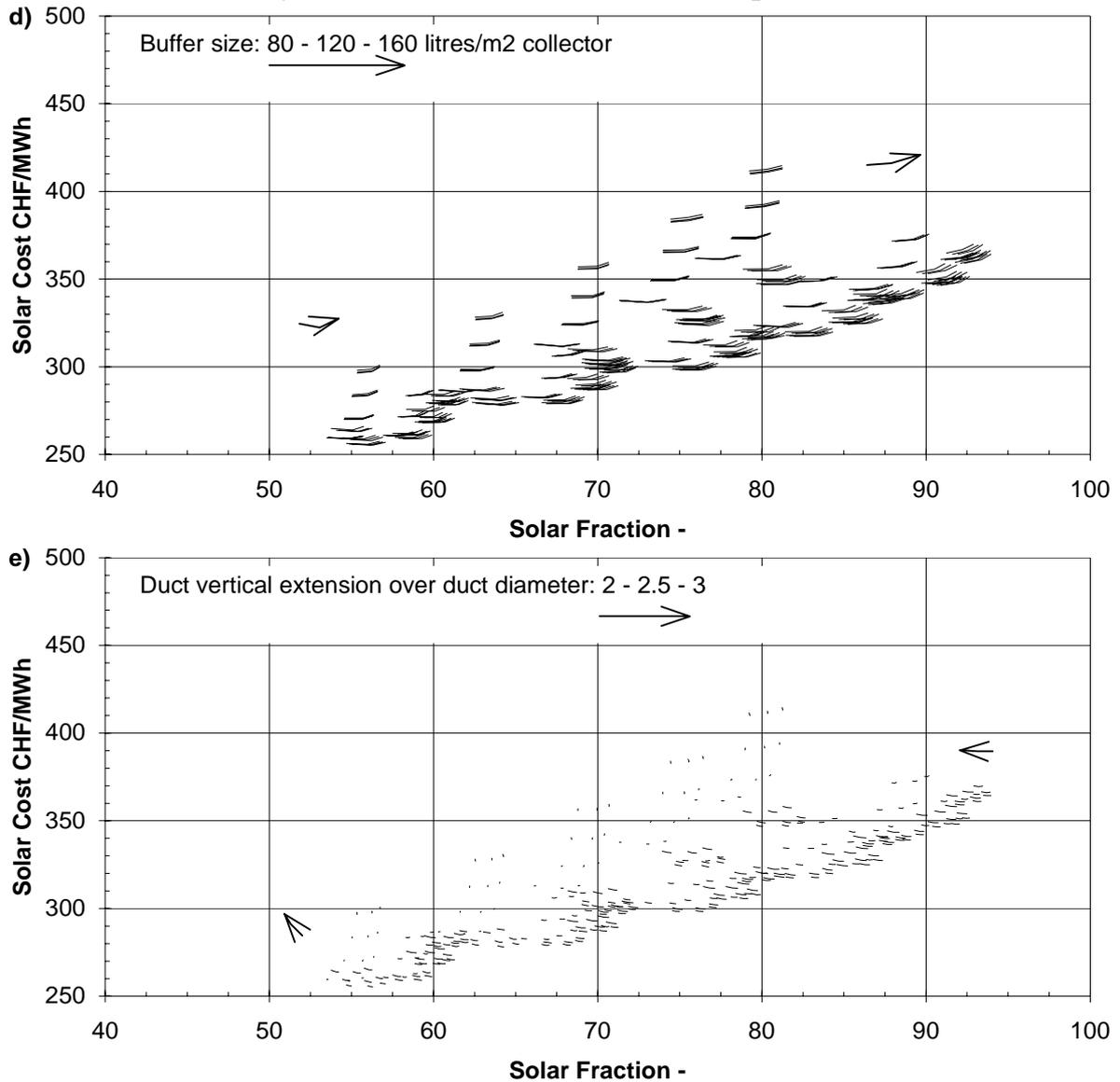
Fig. 8.6d-e: Large heat load, 5'000 MWh/y (50% space heating and 50% domestic hot water); moderate-temperature heat distribution.
