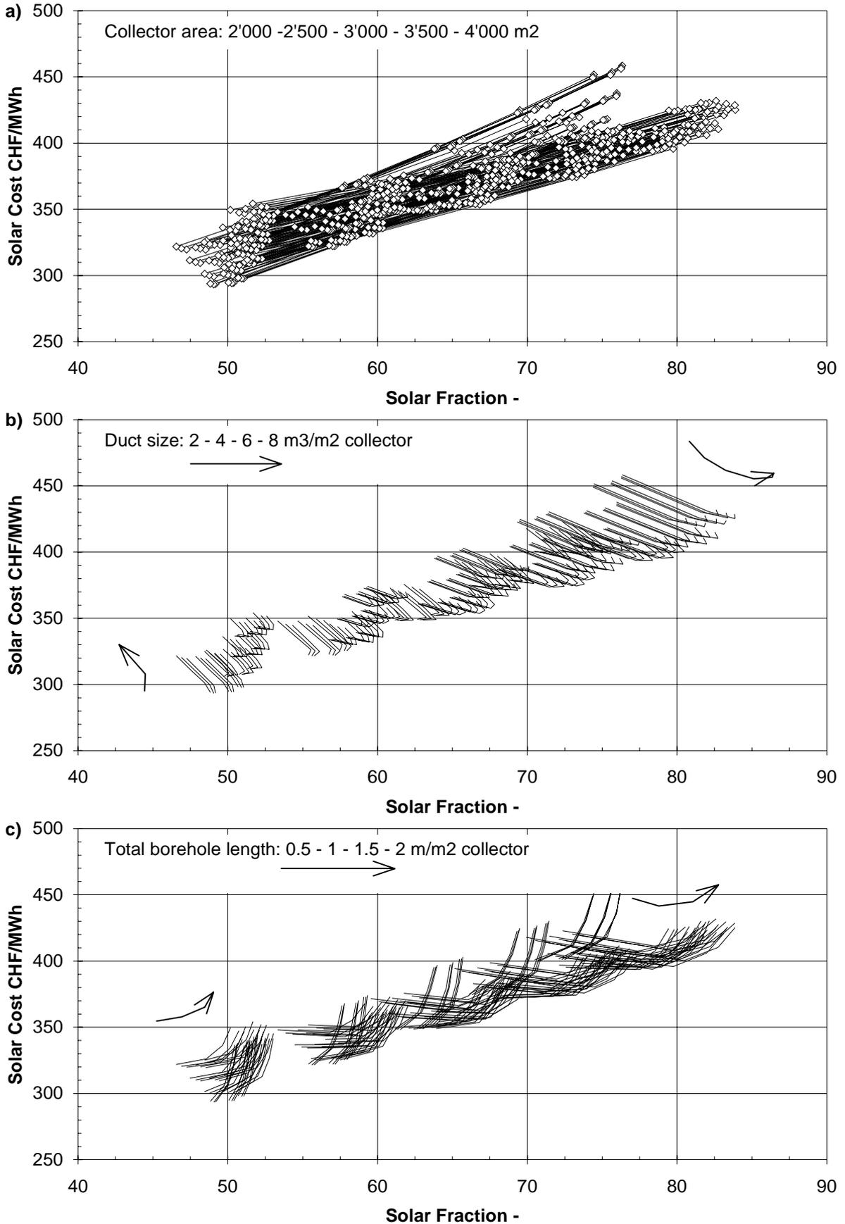
Fig. 8.5a-c: Medium heat load, 1'000 MWh/y (50% space heating and 50% domestic hot water); moderate-temperature heat distribution.
