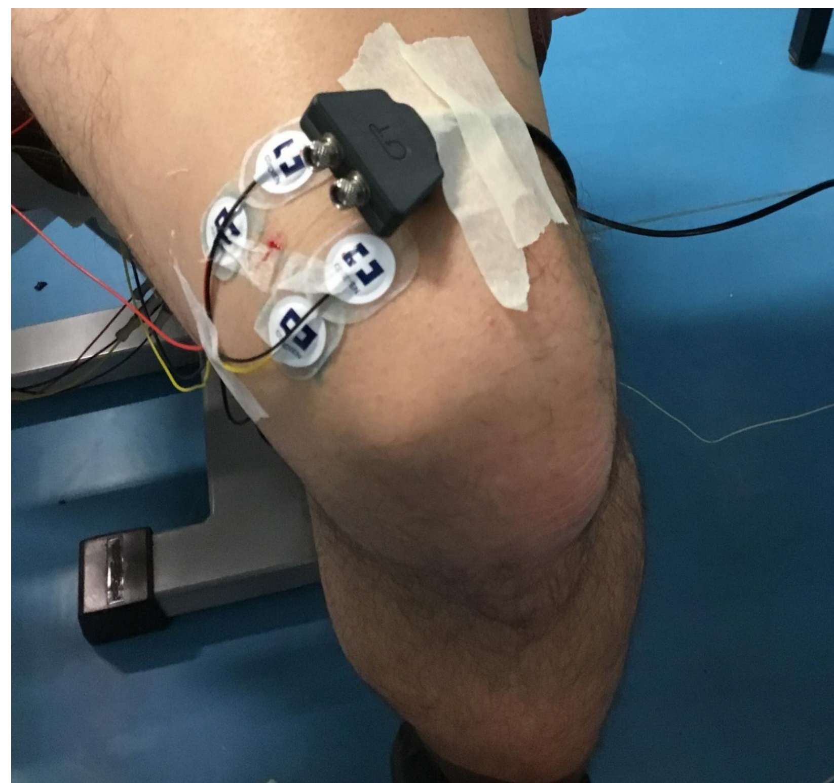
Surface and intramuscular EMG signals were detected from the vastus medialis obliquus, using bipolar and fine-wire electrodes, respectively.
