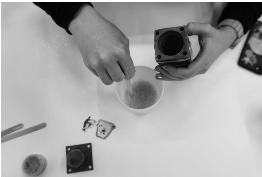
Fig. 2: Participant of 'Make Your Own Menstrual Cup' mixing silicone components with glitter particles and fluorescent pigment.
